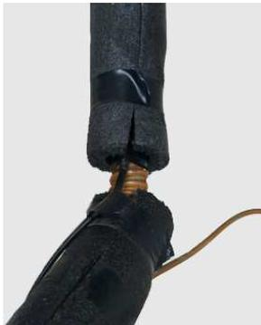
11. Place the other temperature sensor against the hot water outlet pipe of the water heater and tape it securely in place ensuring it is in contact with the copper piping for its entire length. Cover the temperature sensor with insulation.
