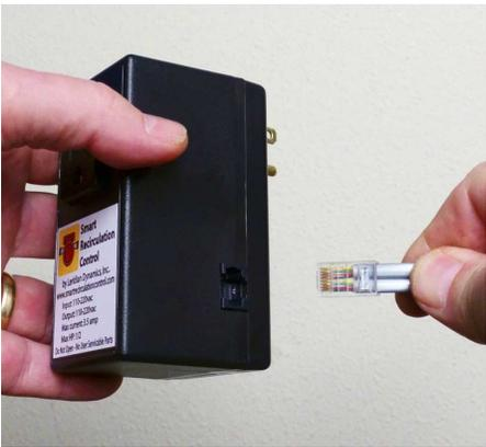
15. Plug the wiring harness into the Smart Recirculation Control 32 via the RJ-45 connector ensuring it snaps in securely.
