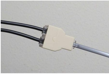
12. Connect the temperature sensors to the wiring harness using the RJ-14 splitter ensuring they snap together securely.
