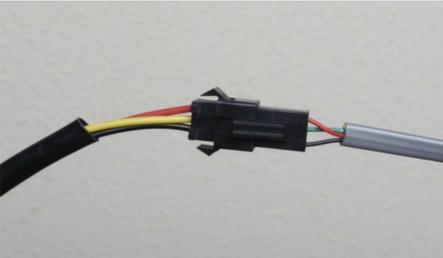
13. Connect the flow meter to the wiring harness via the JST connector ensuring it snaps together securely.
