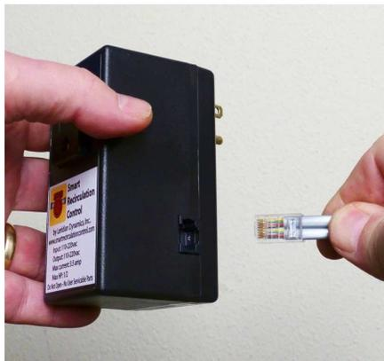
11. Plug the wiring harness into the Smart Countdown Control 32 via the RJ-45 connector ensuring it snaps in securely.
