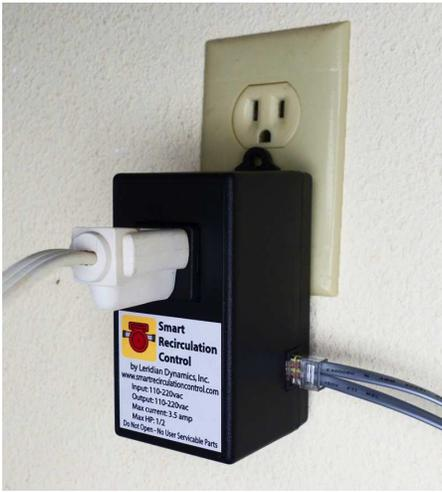
12. Plug the recirculation pump into the Smart Countdown Control 32 and plug the Smart Countdown Control 32 into an electrical outlet.
