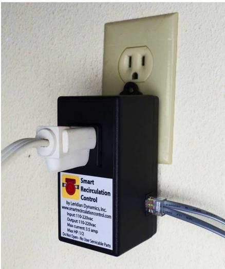
16. Plug the recirculation pump into the Smart Recirculation Control 32 and plug the Smart Recirculation Control 32 into an electrical outlet.
