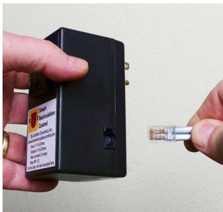
11. Plug the wiring harness into the Smart Thermostatic Control 32 via the RJ-45 connector ensuring it snaps in securely.
